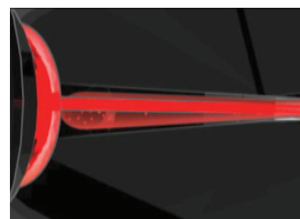
Fig 3. The shadow cast on the photo diode by contaminants in the oil creates a measurable change in the light intensity.
