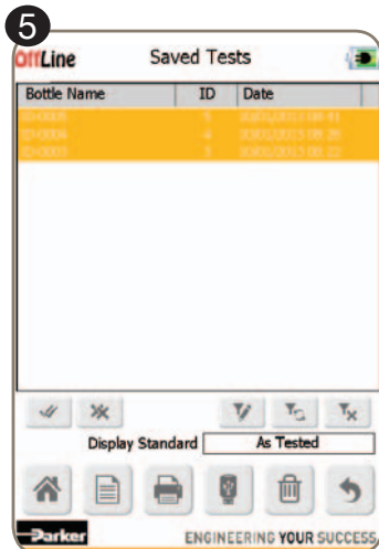
5 Export results: Highlight the test result(s) you would like to export using the stylus.
